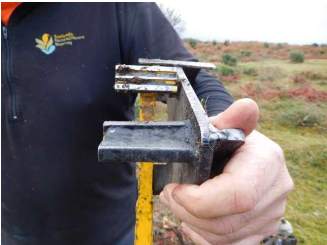
Base of the Tree Popper showing the part which grips the stem
